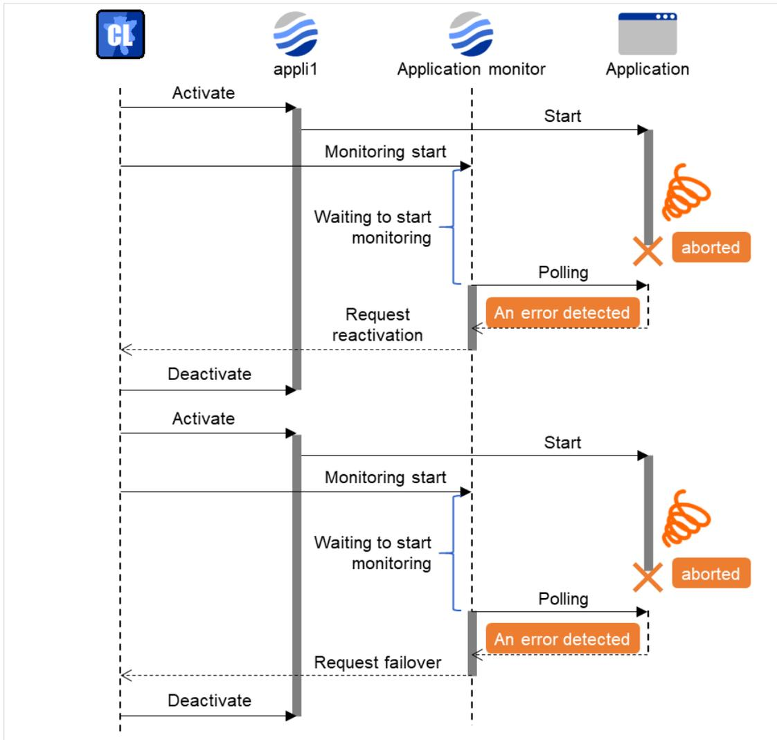
Fig. 7.11: Waiting for a monitor resource to start monitoring (the wait time to start monitoring set to 60 second)
