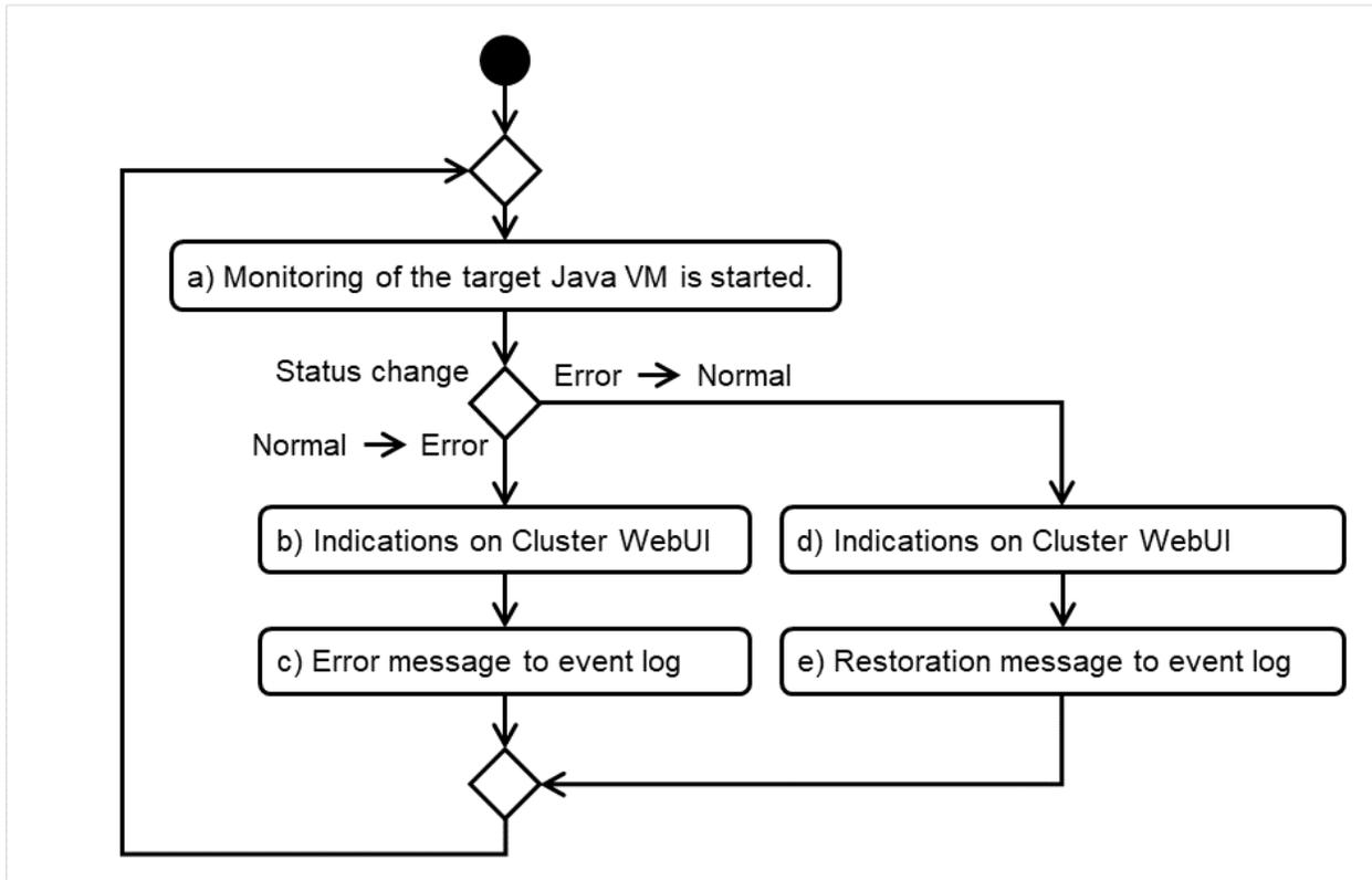
Fig. 5.5: Monitoring flow by the JVM monitor resource
