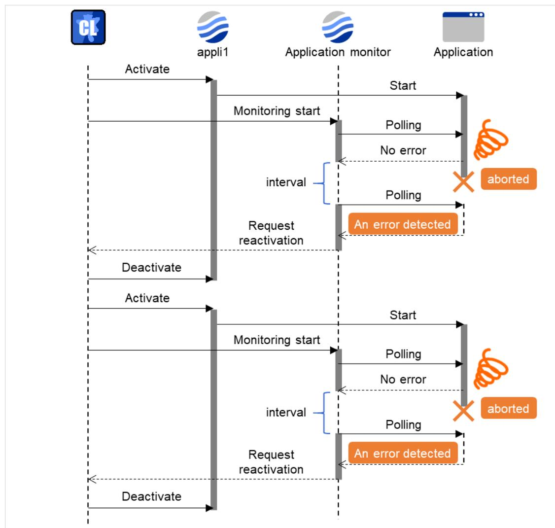
Fig. 7.10: Waiting for a monitor resource to start monitoring (the wait time to start monitoring set to 0 second)
