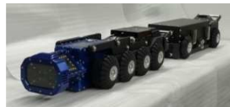
Sewage pipe inspection robot Field tests using actual sewage pipes (Japan Sewage Works Agency, Funabashi City)
