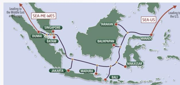
Once IGG is completed, this cable system will not only enhance connectivity between the major cities of Indonesia but it will bridge two other International submarine cables being built by NEC, namely the SEA-US submarine cable system connecting Indonesia to the U.S. and SEA-ME-WE5 submarine cable system connecting Singapore to Europe through the Middle-East. The IGG will empower Indonesia's domestic communication networks, while transforming Indonesia into an international communication hub.
