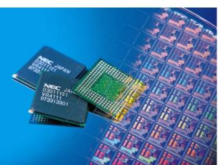
platform. Based on architecture developed by MIPS Technologies, of the United States, the  $V_R$ 4111 was built using a leading-edge 0.25-micron process technology to offer high-speed processing with higher energy efficiency. The result is a twofold improvement in processing speed per unit of power consumption compared with its predecessor.
