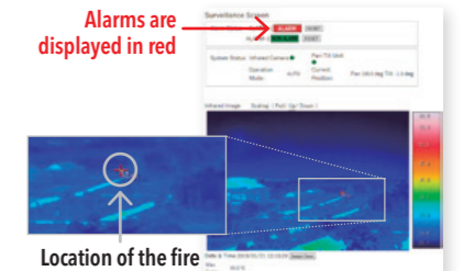
Fire detection screen image using infrared camera
