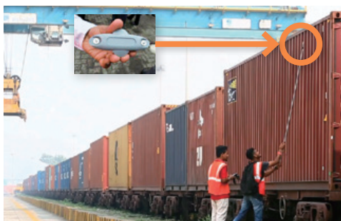
RFID easily attachable to container using magnets
