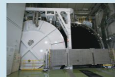
Large-scale space chamber at the Satellite Integration Center
