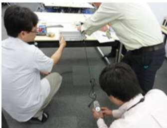
Test of power cord fixing strength (Safety review practice)
