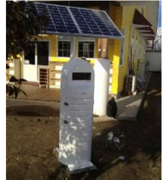
Monitoring post installed in Fukushima Prefecture
