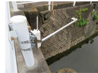
A sensor installed near a riverbank
