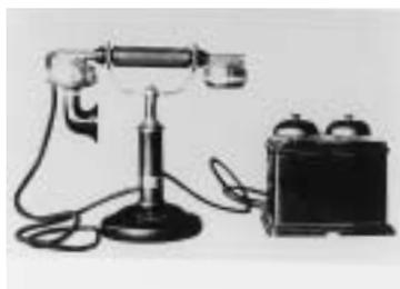
Common-battery switching systems allowed the production of much simpler telephones. The Type 107 telephone introduced in 1924 was officially called the Type 2 common-battery type desk telephone.
