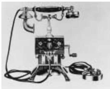
Nippon Electric began producing domestic-made telephone sets not long after its founding. It used various designs, such as this metal Delville-type telephone.
