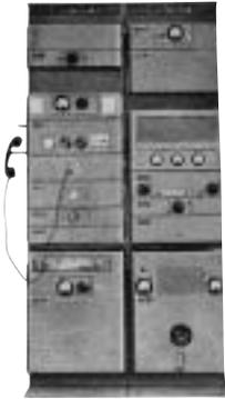
In the early 1930s Nippon Electric began developing power line telephone carrier equipment for transmitting telephone calls. The PL-3, completed in 1947, was an improved version of that equipment.
