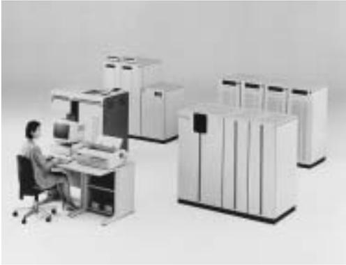
NEC announced in 1994 the Model PX7500 of the Parallel ACOS Series. This series featured reduced cost by using a single-chip CMOS processor, and high speed by using several processors to conduct parallel processing.
