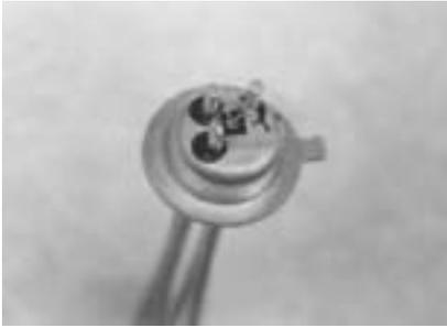
The 2SC33 silicon mesa transistor Nippon Electric developed in 1960 for use in communications was a pioneering product using the diffusion techniques in Japan.
