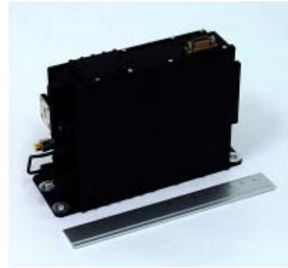
Photo of New Downconverter
