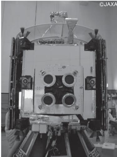
Photo 1 Ion thrusters mounted on the probe.
