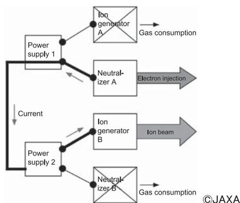
Fig. 10 Scheme of cross-operations of ion engines.
