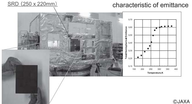
Fig. 5 Mounting of smart radiation device, its temperature characteristic.
