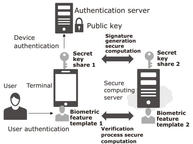
Fig.4 Protection of FIDO-based authentication information using SMPC.
