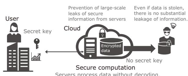
**Fig.1** Prevention of information leaks using secure computation.
