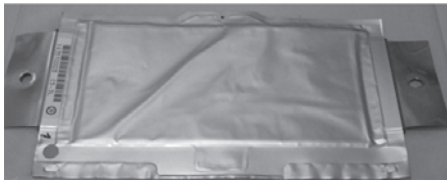
Photo 2 External appearance of the batteries after the external short-circuit test.
