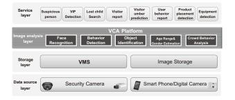
Fig. 1 Concept of the image analysis system.
