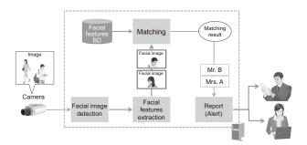
Fig. 2 System image of face recognition.
