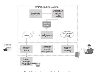
Fig. 3 System image of behavior detection.
