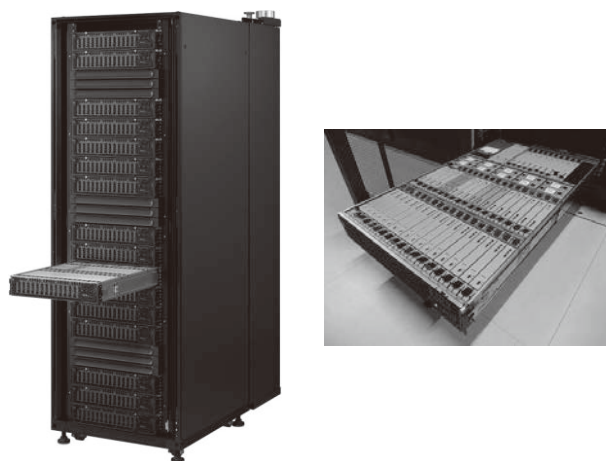
Photo 1 The recently developed micro-modular server.
