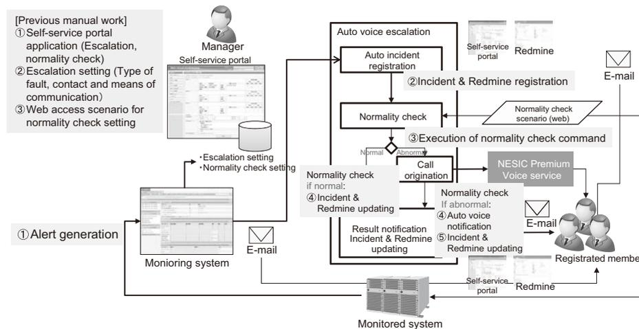
Fig. 3 Configuration of auto voice escalation/normality checks.
