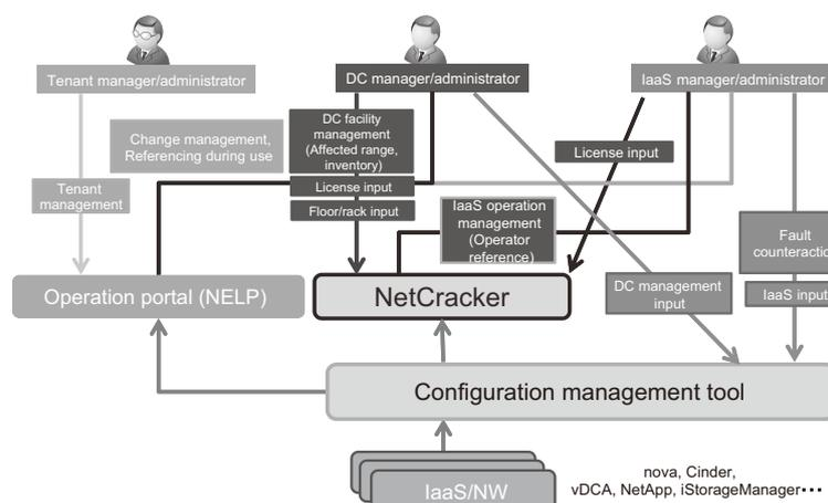
Fig. 1 Configuration of the configuration management application.
