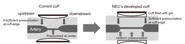
**Fig. 9** Diagram of cuff-edge pressurizing effect improvement and of the size reduction thanks to the stress relaxation structure.
