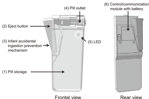
Fig. 7 Drug container with drug dosing alert/management functions.
