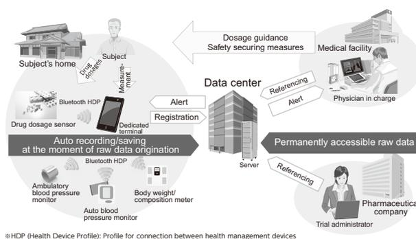
Fig. 10 Diagram of the cloud service for the real-time, online collection of drug dosage detection and vital sign data.
