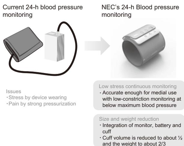
**Fig. 8** Comparison between the current ABPM and the newly developed system.
