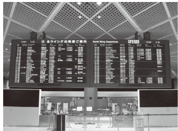
Photo Large display panel using field sequential system.
