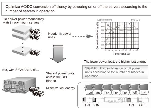
Fig. 3 Optimum power supply operation control (Power ON/OFF according to the number of operating units).
