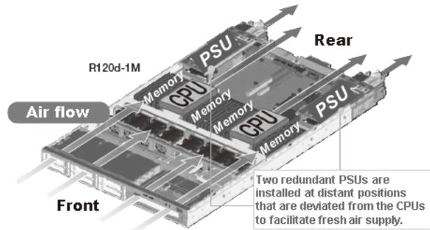
Fig. 7 Cooling structure of high ambient temperature compatible server.
