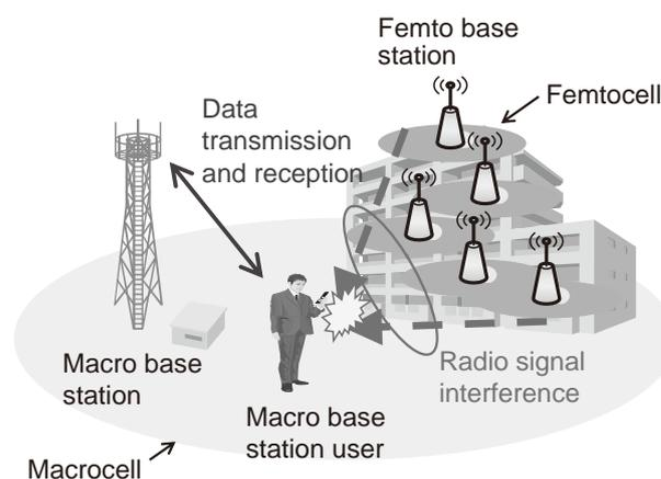
Fig. 1 Radio signal interference between femtocells and macrocells.
