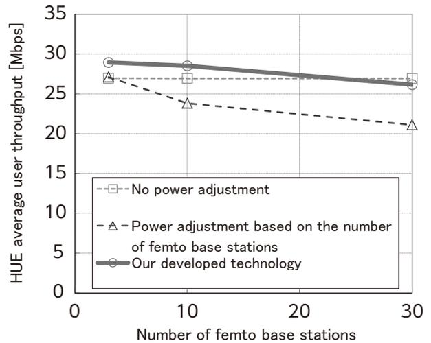
Fig. 4 Properties of the femto terminal (HUE) throughput during times of low data transmission volume at each femto base station.
