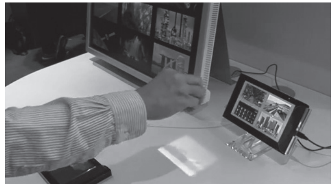
Photo 6 Projected image tracks the hand motion while the selected image is moved to the destination device.
