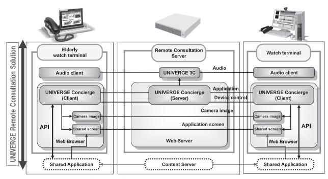
Fig. 1 UNIVERGE Remote Consultation Solution components.
