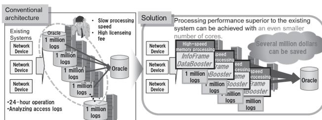
Fig. 5 Case 1: Access log aggregation system.
