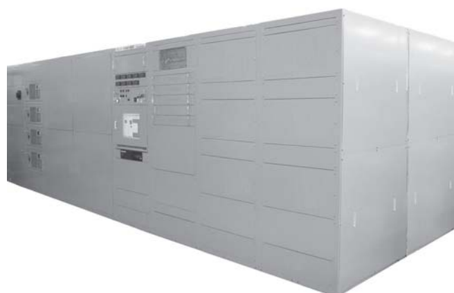
Photo External view of the EV power emulator (300 kW total system).
