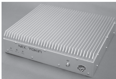
Photo 1 External view of portable reader/writer.
