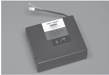
Photo 3 Appearance of 7-series, 2-parallel type standard battery pack.
