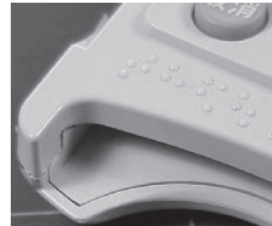
Photo 5 Visible card insertion slot that can show the presence of a skimming device at a glance.
