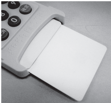
Photo 3 Elimination of clearance for inserting two IC cards.
