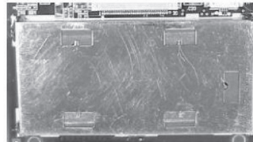
Photo 6 Internal protection with a built-in case shielding for attack detection.
