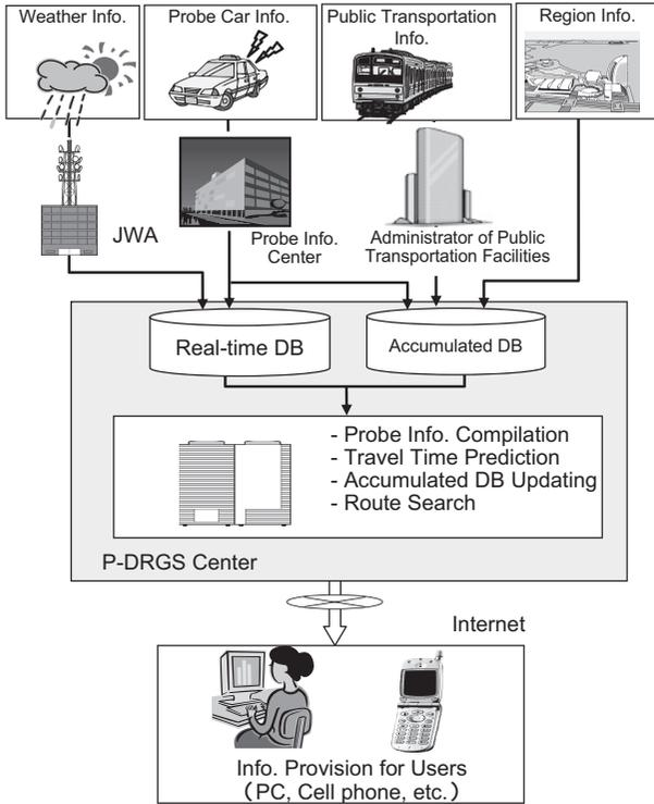
Fig. 1 PROROUTE system configuration.
