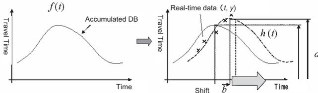
Fig. 5 Transformation from accumulated DB to dynamic DB.
