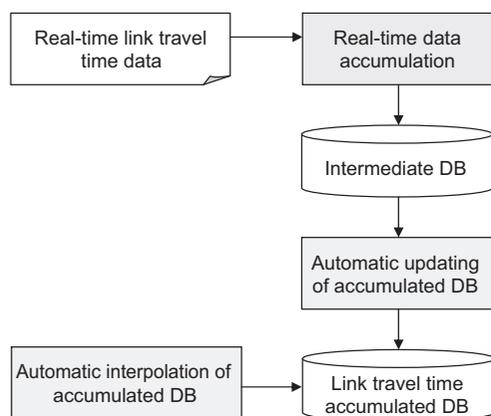
Fig. 3 System configuration of automatic updating of travel time accumulated DB functions.
