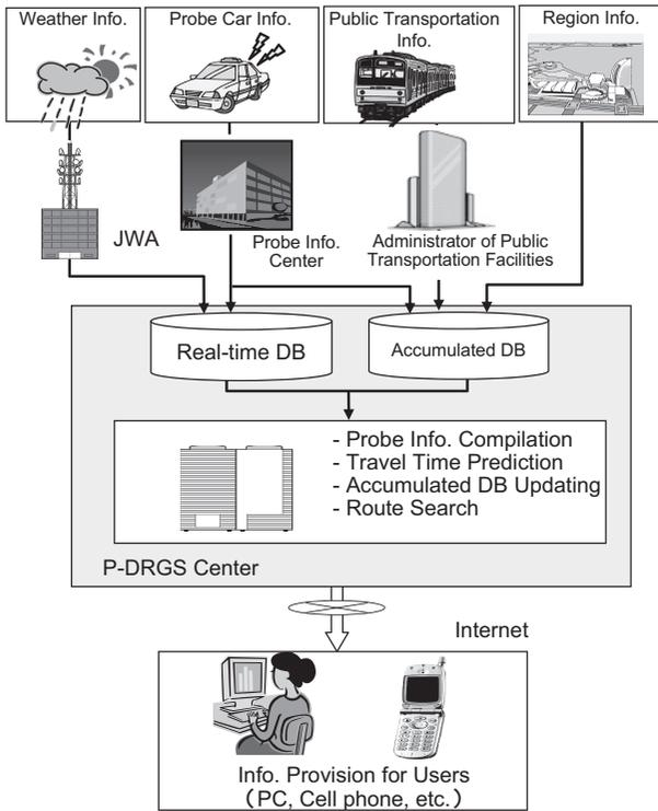
Fig. 1 PROROUTE system configuration.
