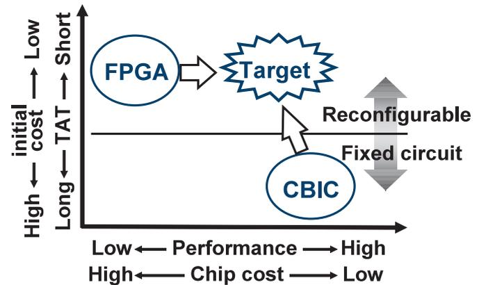
Fig. 1 Comparison between CBIC (Cell-based IC) and FPGA (Field programmable gate array).
