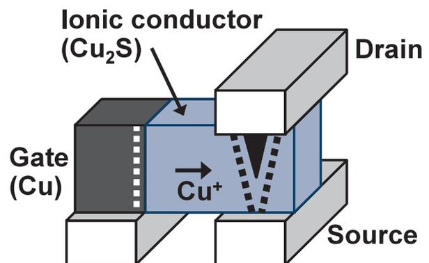
When positive voltage is applied to the control line, metal is precipitated between two metal wires via electrochemical reactions. Negative voltage results in precipitated metal dissolving in the solid electrolyte.
