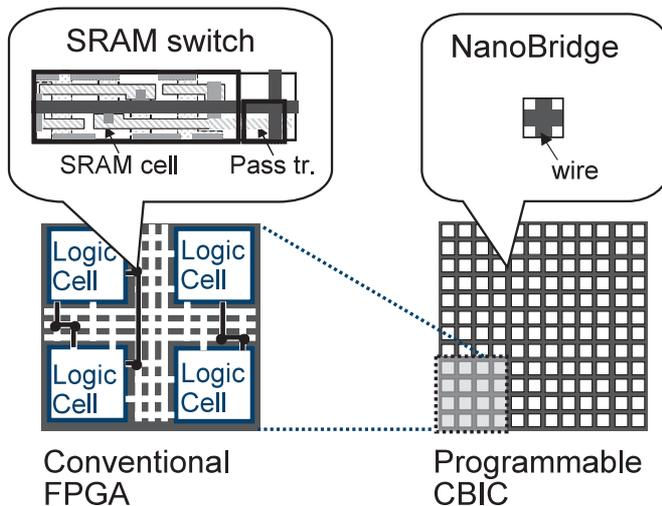
Fig. 2 Conventional FPGA and the proposed programmable device. The white region represents the logic area and the gray one represents the switch area. When NanoBridge technology is applied, a small logic cell can be used and the logic cell usage efficiency can increase.
