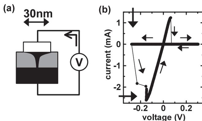
Fig. 3 Left: Schematic view of NanoBridge composed of a  $\text{Cu}_2\text{S}$  film sandwiched between Cu film and top electrode. Right: Current-voltage characteristics of NanoBridge with a  $0.03\mu\text{m}$  contact size.
