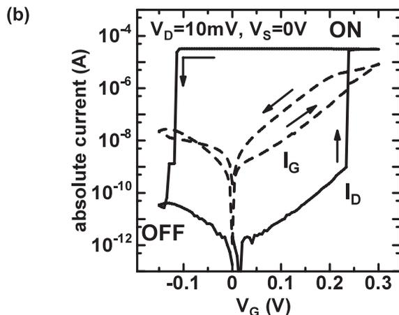
Fig. 6 (a) Operation of three-terminal NanoBridge. (b) Drain current ( $I_D$ ) and gate current ( $I_G$ ) with changing gate voltage ( $V_G$ ).
