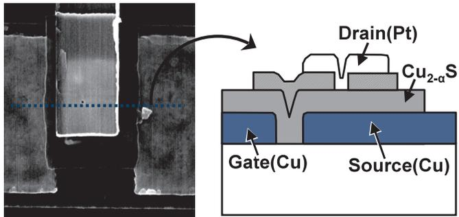
Drain electrode connects to  $\text{Cu}_{2-a}\text{S}$  via  $0.2\mu\text{m}$ -diameter hole in calixarene (negative electron beam resist).
