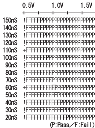
Fig. 4 Example of Shmoo plotting (horizontal axis represents power supply voltage, while vertical axis represents test rates. The lower the coordinate the faster the operating speed. The red color marks the borderline between pass and fail.)
