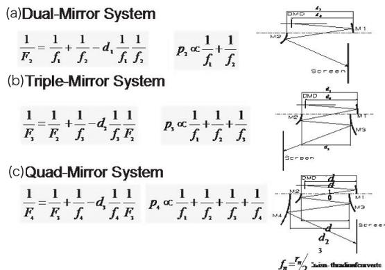
Fig. 2 Examples of mirror configurations and their focal distances and aberrations.
