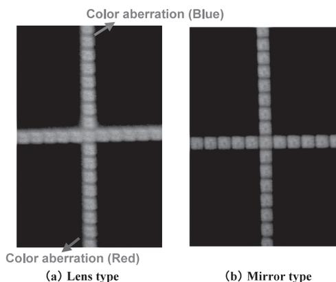
Fig. 6 Examples of the color aberrations of a refractive lens and a reflective lens.
