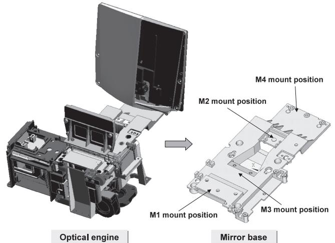
Fig. 4 Example of the optical engine configuration and base plate.
