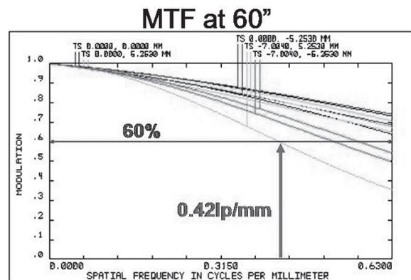
Each line of graph shows MTF curves at 5 grid points in right half image area. Calculation wavelengths are 650, 546 and 460nm.
