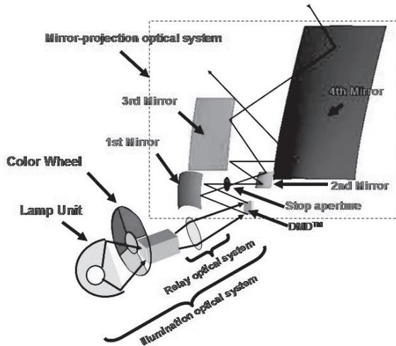
Fig. 3 Diagram of optical configuration model.
