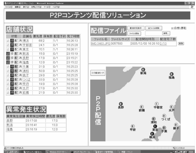
Fig. 7 A screen representing a management server display shows locations of failure on the network.
