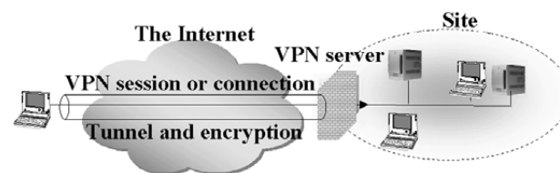
Fig. 6 Principle of tunneling protocol.
