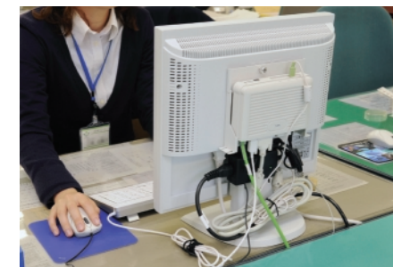
Thin client terminal is placed behind a display monitor and provides better system performance and increased productivity.
