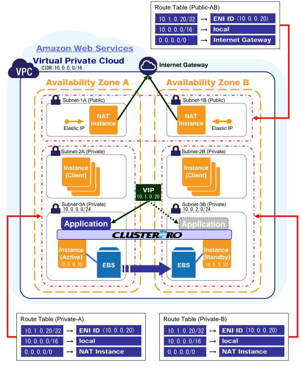
Figure 3-1 System Configuration: HA Cluster Based on VIP Control
