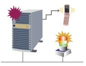
Alert email can be sent to the administrator when a failure or failover occurs. In addition, the status of servers can be visually checked anytime through network warning lights.
