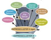
In addition to monitoring to determine whether the various applications in a cluster are alive or dead, the status of the applications including hang-up and abnormal response can be monitored. Seven types of agents are available for each supported application.
