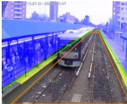
Monitor platform to alert when someone intrudes railway path
