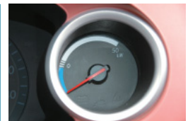
Meter shows battery power in kW
