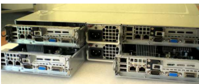
NEC HPC 2812Rb-2: hot-swappable PSU and Server-Blades
